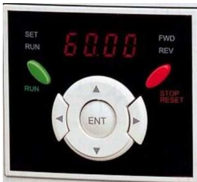
[Rys. 1] Inverter Panel
