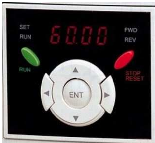
[Rys. 1] Inverter Panel
